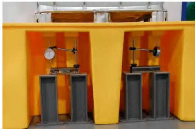
Measure the deflection of the pallet
